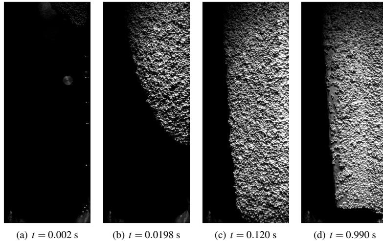
Figure 2: Snapshots of the free surface flow of glass beads immersed in a kaolin-water dispersion at  $20g$  and slope angle of  $30^\circ$ . The time of each snapshot is relative to the time of release. A detailed description of the Centrifuge experimental model and its results is presented in Ref. [1]
