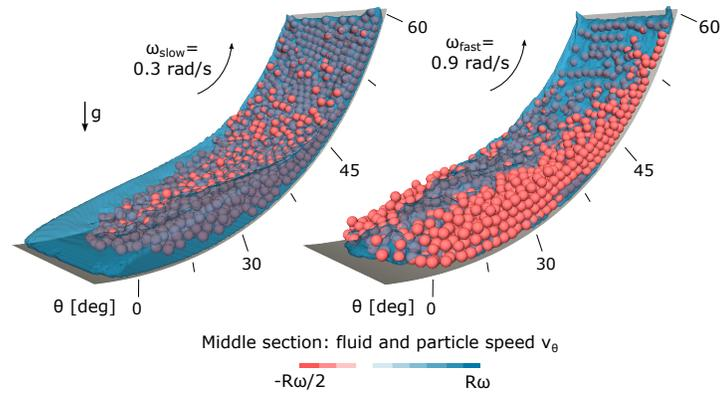
Figure 1: Snapshots of the DEM-LBM simulations (particle content of 31%). The formation of a granular front is induced by an increase in the angular velocity of the drum. A detailed description of the DEM-LBM method and its implementation is presented by Leonardi in Ref. [2].
